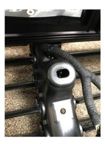
NOTE: Make sure wiring is routed down the correct side, as shown in the picture above.
