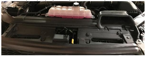
2. Disconnect the two wiring connectors, and the quick-disconnect for the fluid washer fluid hose. Then remove the four bolts securing the front grille, shown below.
